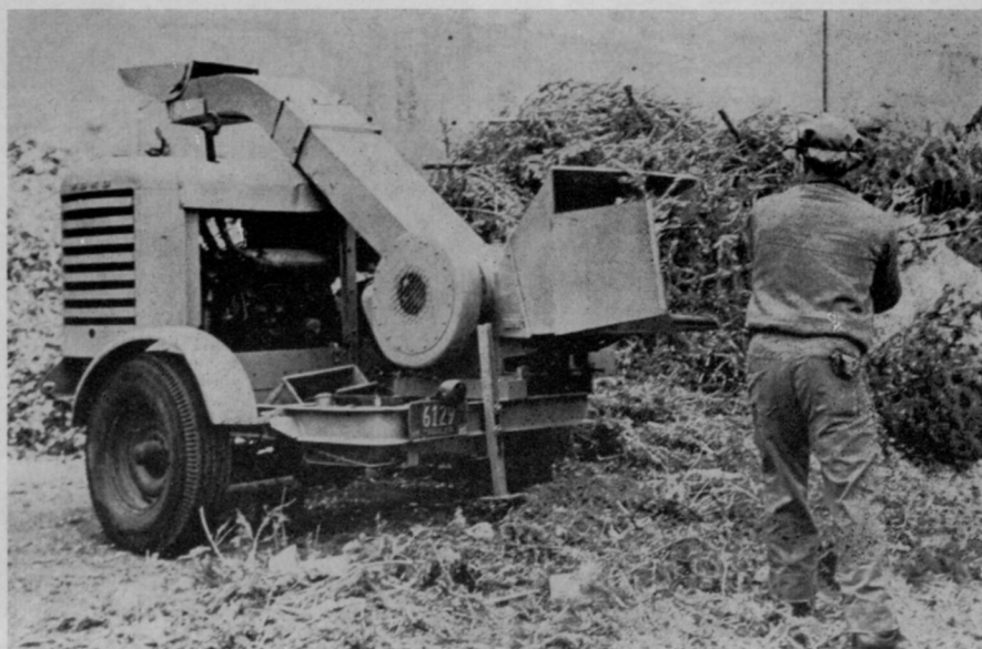
Christmas tree disposal problems are being simplified nationwide by use of wood chippers. New York City's Sanitation Department uses Fitchburg Brush Chippers such as the above to reduce trees to chips. Once trees are put through chippers, refuse is hauled to incinerators and burned. City last year required 70 trucks just to deliver trees to chippers. In other areas, chips are used for mulch, and one mid-west city reported it cut disposal costs by one-third by chipping trees. Prior to use of chippers, tree disposal created problems with bulk alone, besides damage to incinerators from tree spikes.
