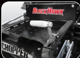
OCDC – Foot-operated discharge chute to control grass clippings
