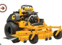
for Wright's line of Stander ZK zero-turn mowers. The 72-in. Stander ZK's wider cut, push-button deck lift, powerful engine options, mowing speed of 12.5 mph and fully independent left/right hydro systems all contribute to the mower's improved productivity, the company says. Reinforced wheelie wheels and elastomer bumpers for progressive ride control help the mower hug the ground on all terrain.
