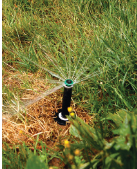
The Alpenglow team uses rotary nozzles (above) and conducts an irrigation system installation (right).
