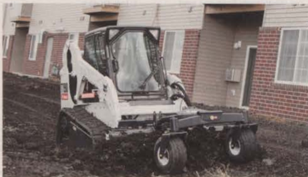
Bobcat T190 compact track loader with soil conditioner
