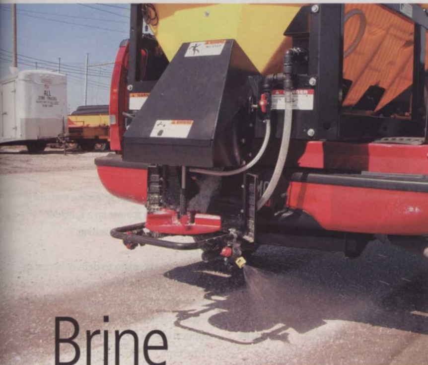
A V-box style spreader has hoses leading to the tank that holds the brine near the truck's cab. The nozzles spray in a fan pattern directly onto the driving surface.
