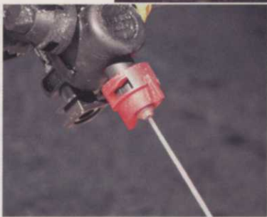
A pre-wetting system can be used to wet the spreading material in the chute before it hits the distribution spinner on a spreader. (Left) A closeup shot of the pencil-spray nozzle setting.
