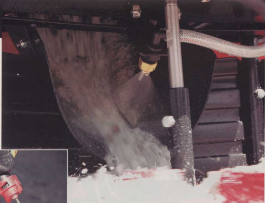
A pre-wetting system can be used to wet the spreading material in the chute before it hits the distribution spinner on a spreader. (Left) A closeup shot of the pencil-spray nozzle setting.
