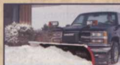
Full-featured conventional plowing with the C-Plow in push position.
