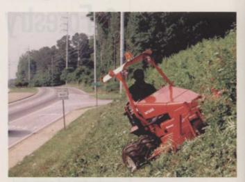
confidence provided by a 38-hp diesel and true zero degree-turning radius makes the Kut Kwick SSM38-72D the obvious choice for your entire slope mowing needs.
