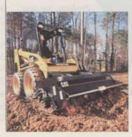
trenching and digging tasks in tight spaces. The newest models feature variable displacement hydraulic pumps for unmatched ability to dig through tough conditions. A variety of work tools equips these machines to do more than digging.
