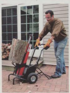
hydraulic pressure to split logs up to 20-in. long and 12-in. wide. The dolly carriage design makes maneuverability easy, indoors or out.
