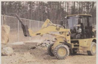
to handle a wide range of work tools. Auxiliary hydraulic flow of 22 gpm enables the loader to operate productively with hydromechanical work tools such as tillers, trenchers, snow blowers and cold planers.
