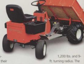
PowerWolf's safe, stable and vision-friendly design features an electric front dump. The steering wheel combined with low-maintenance, hands-free automatic transmission promises safety and ease of use.
