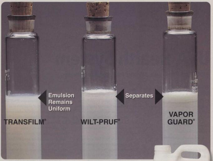
Can you really see a difference in anti-transpirants? The photo above shows that Transfilm (left) remains emulsified while leading competitive products have separated 48 hours after mixing. Separation can cause spray tank problems as well as uneven coverage. Transfilm's stable emulsion provides even coverage that resists cracking and peeling. For complete test details, see our web site at www.pbigordon.com.
