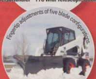
Skid-Steer Loader with Snow V-Blade
