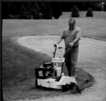
Redefine bunker edges
