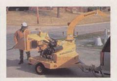
thick cutter disc for more cutting inertia, and an improved variable speed hydraulic system that delivers 20% more torque to the feed roller. Three engine options are available, including a 20-hp Honda, a 25-hp Kohler Command, and a 23.5-hp water-cooled Perkins diesel.
