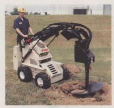
crews do more work faster, and with fewer personnel. A 25-hp Kohler engine generates a hydraulic flow rate of 13.4 gpm. Full power is delivered to wheels and tools at same time. Oil cooler is standard. Quick-change feature allows attachment changes in less than one minute. Over 30 attachments are available, including trencher, tiller and box rake.
