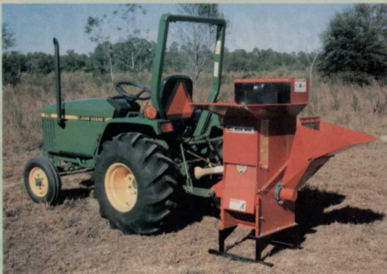
Bush Hog chipper/shredder mounts by 3-point hitch to tractor with at least 18 hp. Shredder knives and chipper knives are machined from tool steel.
