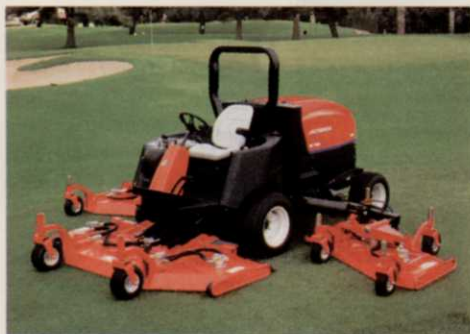
Jacobsen HR 9016 Turbo has a 16-foot cutting width and 8.5 mph speed.
