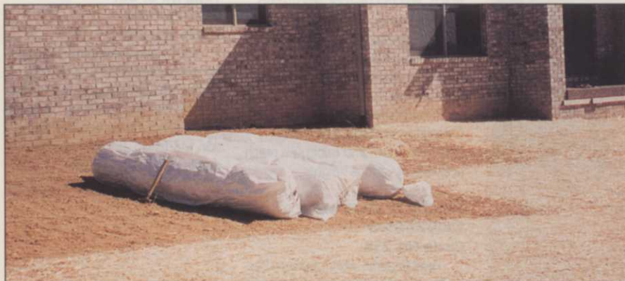
A 60 square-yard roll of wheat straw blanket weighs only 30 pounds.
