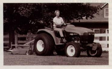
diesels, have hydrostatic power steering and are equipped with wet-disc brakes.
