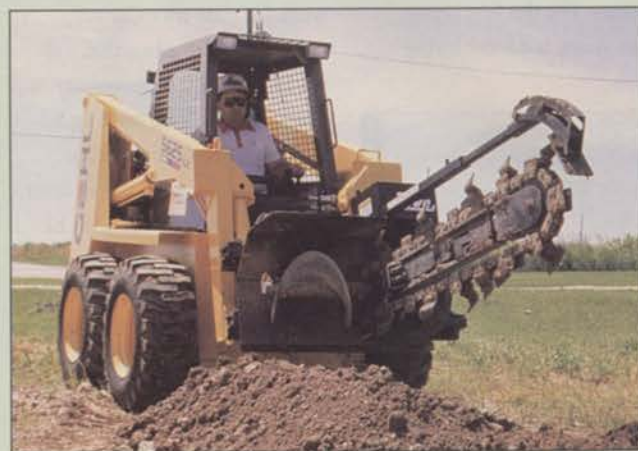
Gehl trenchers feature a heavy-duty digging chain.
