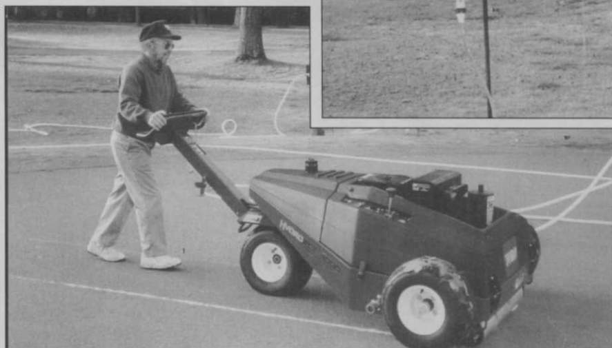
Harold Edgerton has used a Dosatron/HydroJect hook-up for more accurate injection of wetting agents and to dry out wet golf greens. The Dosatron injector (inset) is self-priming. It pulls the wetting agent into the mixing chamber where it's accurately blended with water flow.
