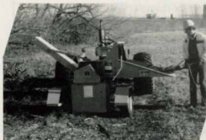
Model 12 — PTO, 3 pt. hitch or tow-type, 7" capacity, 500 lb. drum.
