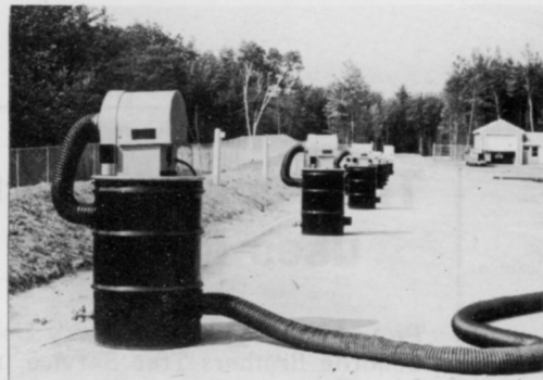
Plastic pipes hooked up to a holding tank with a fan draw liquid waste and odors from compost piles.
