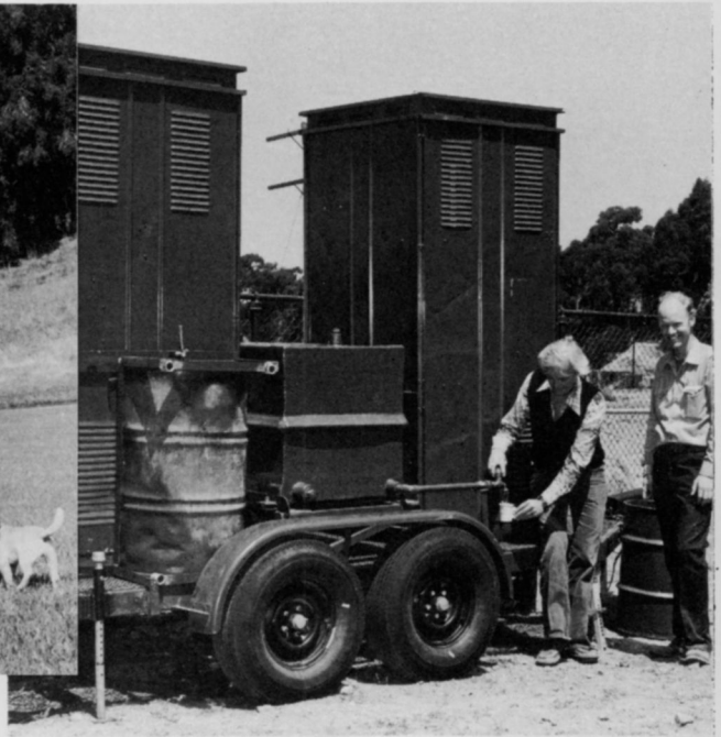
Special toilet trailers for back country campouts eliminate road damage by heavy pumpout trucks servicing out of the way latrines. The trailer carries water, barbecue pits, garbage cans, and two chemical toilets.
