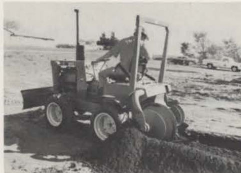
30-HP Model V30 — Trenching capabilities to 18" width, to 6' depth
