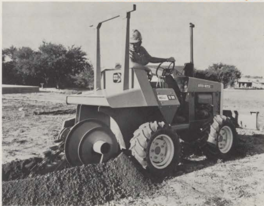
30-HP Model R30 — Trenching depths to 6' plus Modularmatic versatility
