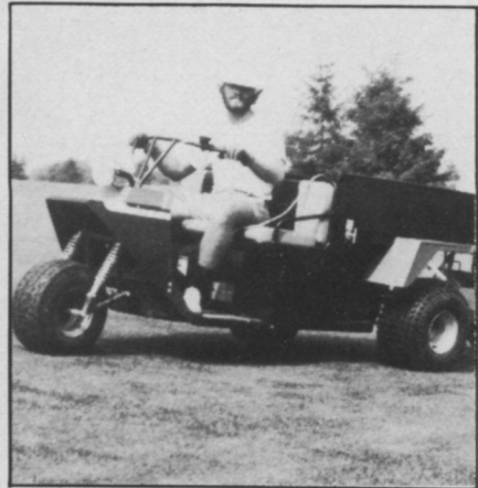
QUARTER HOUR is a new utility vehicle from Promark with a counter-balanced dump bed which holds 500 lbs.
