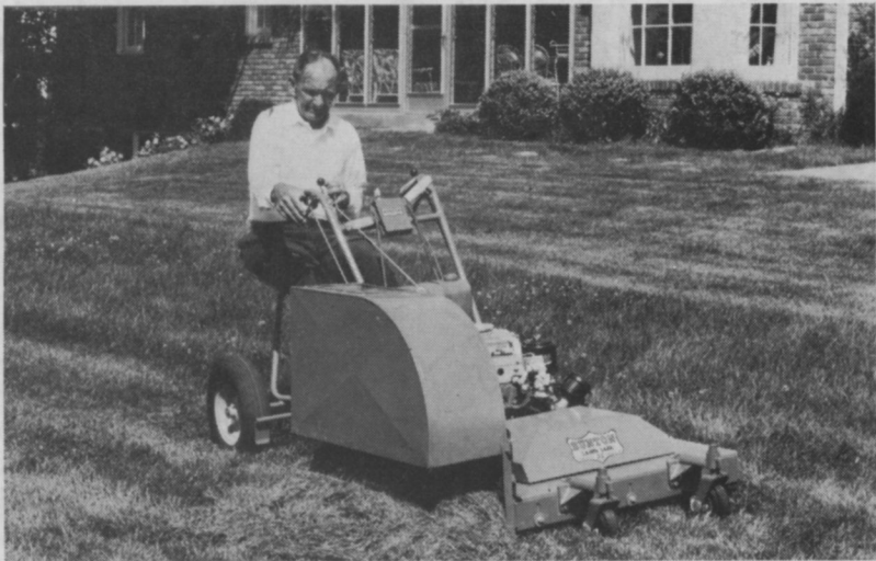
Bunton Co., Louisville, Ky., offers options for its "Lawn Lark" mower units, such as the grass catcher attachment, shown above, operated by handle control. Clip-pings can be dumped into windrows or hopper can be emptied directly into containers. Another option shown is Bunton's easily installed riding sulky that allows an operator to ride open areas and medium grades. Standard features of Bunton's "Lawn Lark" line include finger-tip power steering, 7 forward speeds and adjustable cutting heights. For more details circle (706) on reply card.
