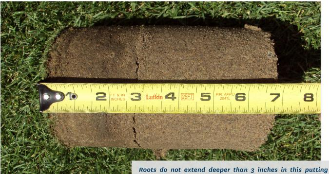
Roots do not extend deeper than 3 inches in this putting green because of a disparity in moisture retention between the surface layer and the original construction mixture.
