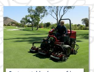
Front-mounted brushes on a fairway mower will stand up turf before cutting and, when routinely used, will improve the uniformity of the playing surface.
