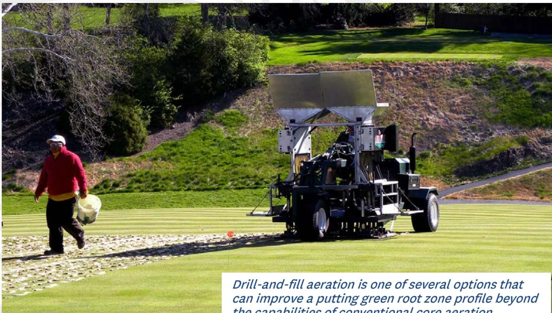
*Drill-and-fill aeration is one of several options that can improve a putting green root zone profile beyond the capabilities of conventional core aeration.*
