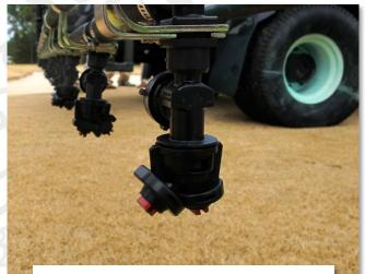
Measuring nozzle output helps ensure uniform product distribution. Nozzles that are significantly worn need to be replaced.
