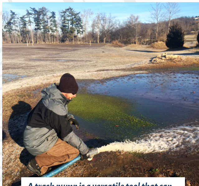
A trash pump is a versatile tool that can be modified to wash silt from flooded turf. (Photo courtesy of Greg Parkinson, Tapawingo National Golf Club)
