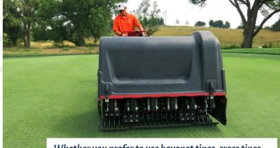
Whether you prefer to use bayonet tines, cross tines, needle tines, or a spiker, venting is vital to sustaining healthy turfgrass during stressful weather.
