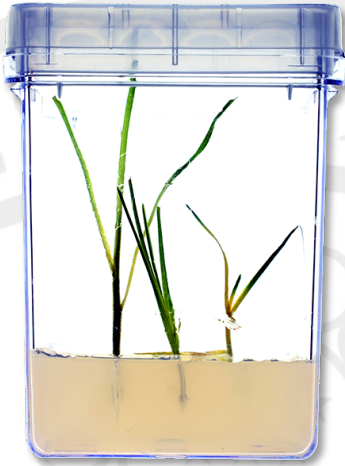
A polycarbonate plant culture box used to diagnose annual bluegrass ( Poa annua ) resistance to herbicides in agar culture.
