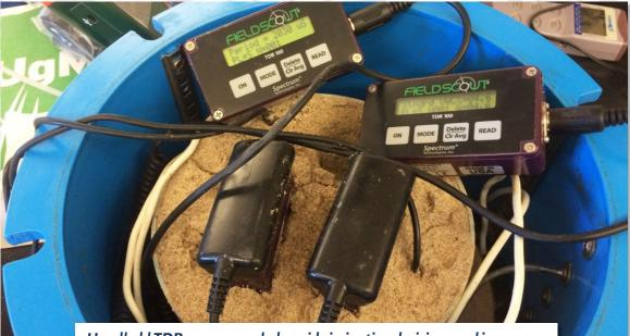
Handheld TDR sensors can help guide irrigation decisions and improve playing conditions, but special calibration may be needed in saline soils.
