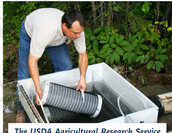
The USDA Agricultural Research Service evaluated cartridge filters installed on drainage lines to reduce the amount of phosphorus entering a lake.
