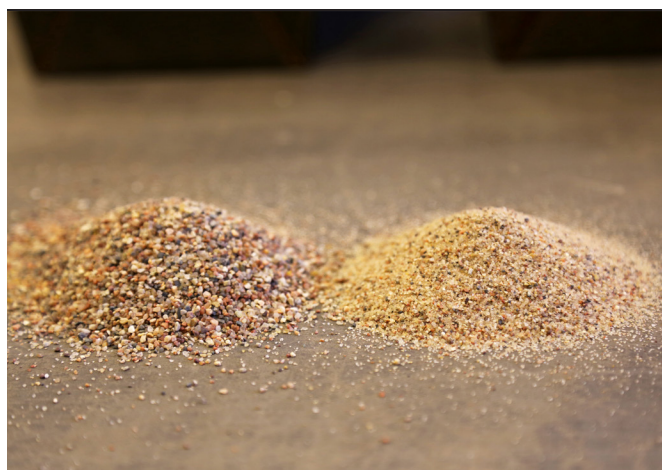
THE SIZE AND SHAPE OF ROOTZONE SAND PARTICLES WILL HAVE A SIGNIFICANT IMPACT ON PUTTING GREEN PERFORMANCE.
