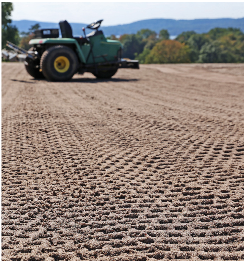
A MECHANICAL BUNKER RAKE WITH KNOBBY TIRES CAN IMPROVE SEED-TO-SOIL CONTACT.
