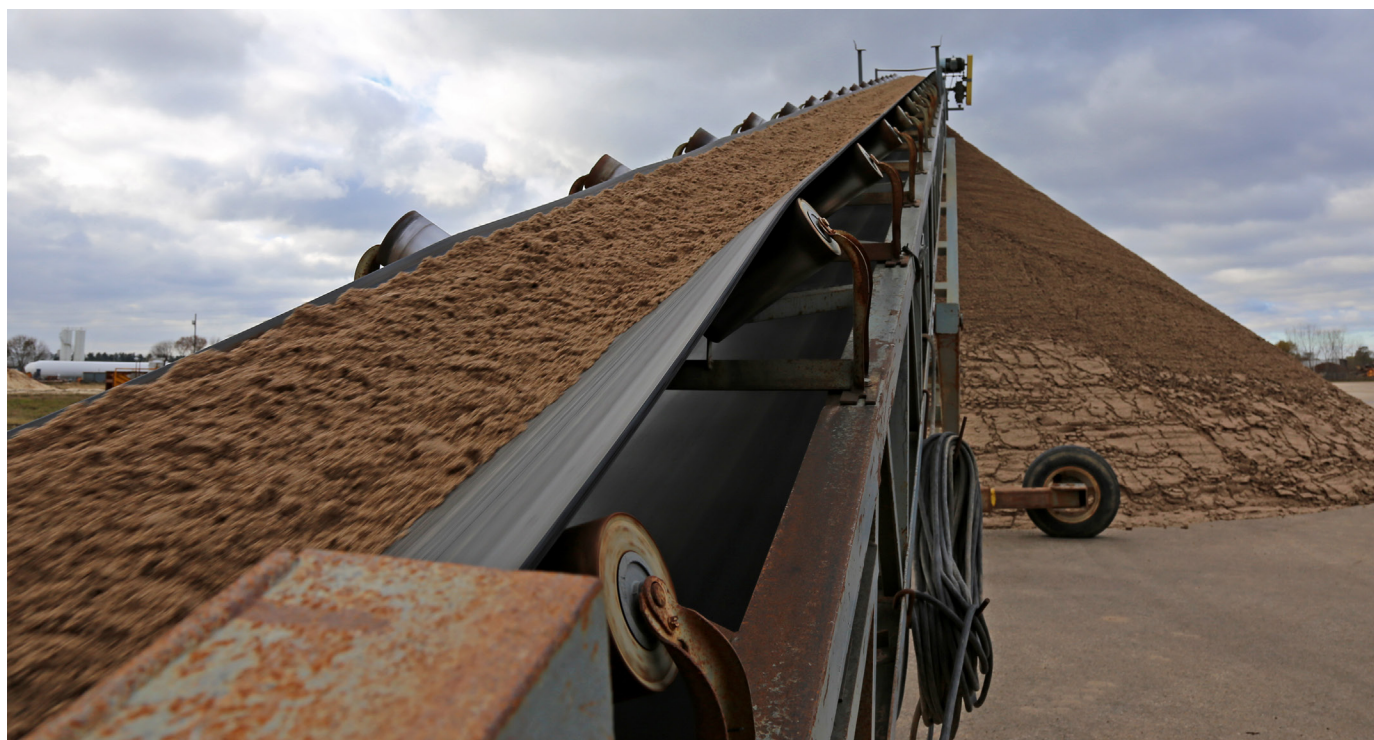
BLENDING THE ROOTZONE MATERIALS AT THE SAND PLANT PROVIDES NUMEROUS ADVANTAGES OVER BLENDING AT THE CONSTRUCTION SITE.
