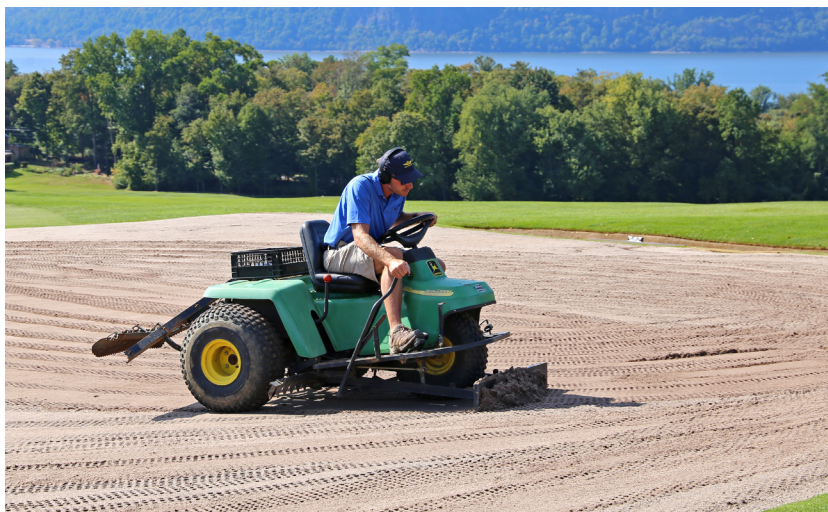
A MECHANICAL BUNKER RAKE CAN BE VERY HELPFUL FOR SMOOTHING THE PUTTING SURFACE AND FINE TUNING THE FINISHED CONTOURS.
