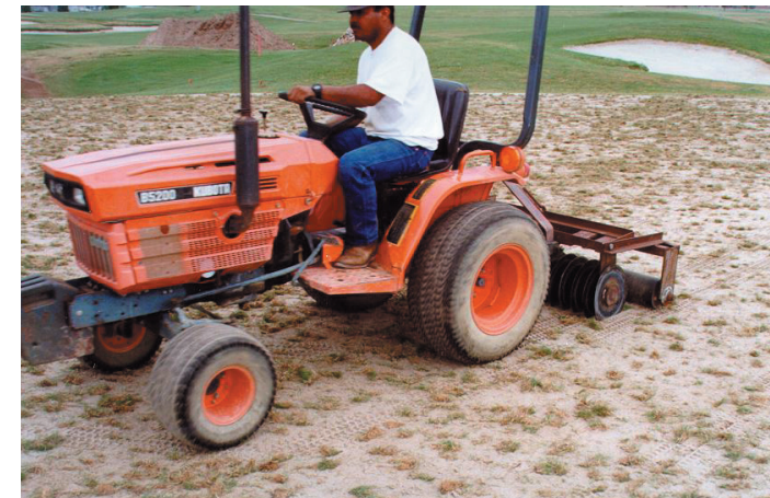
Bermudagrass sprigs should be "cut" into the rootzone with a small, straight disc.
