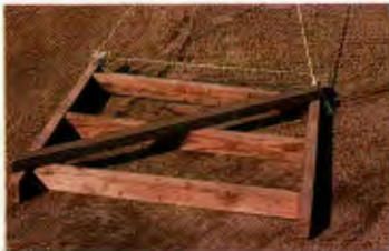
"Floating Greens" provides a smooth finished grade. A light golf cart can mechanize this job.
