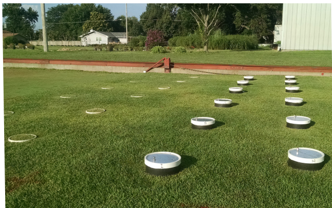
Twelve static chambers (right side) were used for sampling N 2 O across 36 plots on each measurement date.
