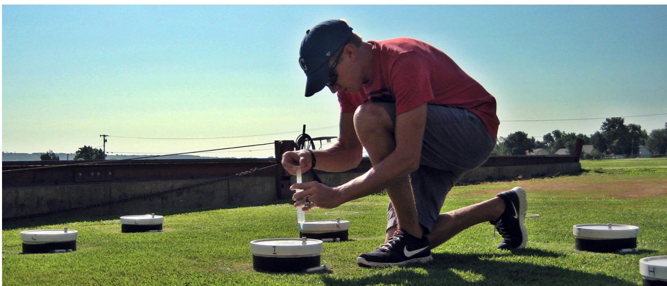
A nitrous oxide (N 2 O) measurement date during the summer using static chambers mounted on base collars in the soil. A single measurement date required 20 hours.
