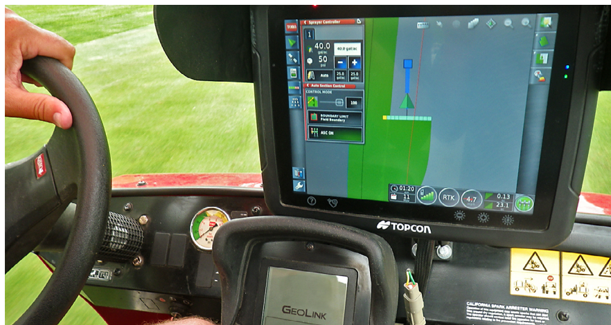
GPS-guided sprayers allow the operator to map target areas and track which locations still need to be treated during an application.
