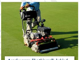
A reel mower, like this walk-behind unit, cuts at fractions of an inch to create silky-smooth putting surfaces.
