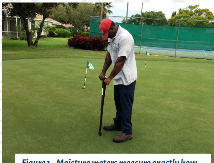
Figure 1 - Moisture meters measure exactly how much water is in the soil at any given time and help the staff determine how much irrigation to apply.
