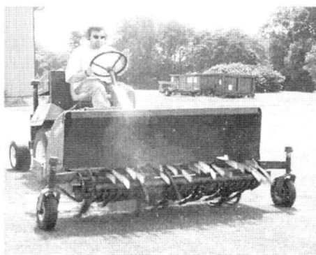
Figure 1. A wear simulator was developed using a modified Sweepster unit. The steel and nylon brush on the Sweepster was replaced with rubber paddles. The modified Sweepster was mounted on a Toro Groundsmaster.
