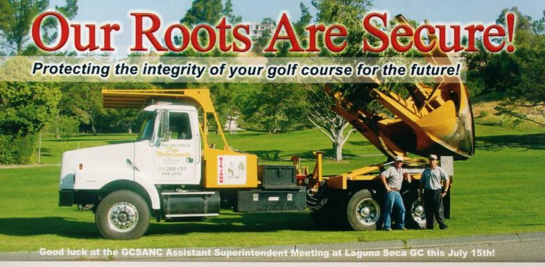
**J. Arnaz Tree Movers** owns state-of-the-art Tree Moving Equipment including, 65" and 90" hydraulic tree spades that allow for the transplanting of any tree without damaging the fragile root system...successfully!!!
