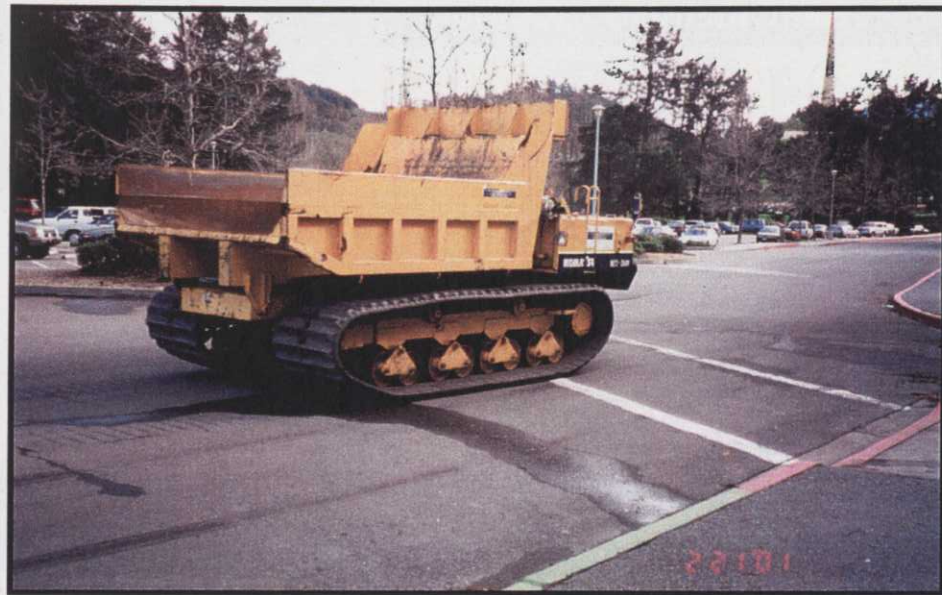
LGP Vehicle On Street – Marin Civic Center
