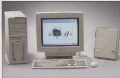
Central control system offers automatic ET adjustments, two-way command verification and Flow Optimizer.
