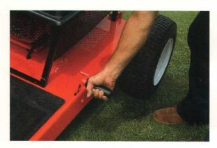
Retractable wheels, with soft turf tires, lower easily for quick transport between greens.
