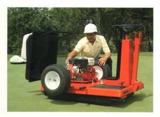
Engine is easily accessible and rubber-mounted to minimize vibration. Leak-proof drip plate prevents hydraulic fluid damage.
