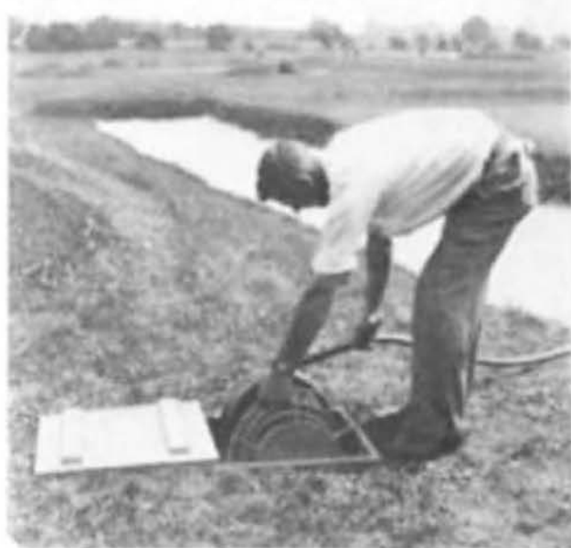
Invisibe Hose Reel provides convenient storage and lowers labor and hose costs.
