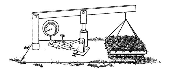
Figure 1: Hydraulic pump apparatus for lifting sod pieces.
