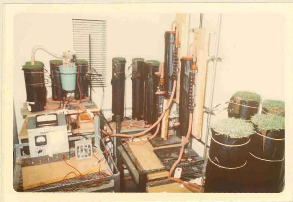
Figure II-4. Setup of Experimental Equipment in the 15°C Controlled Climate Room.
