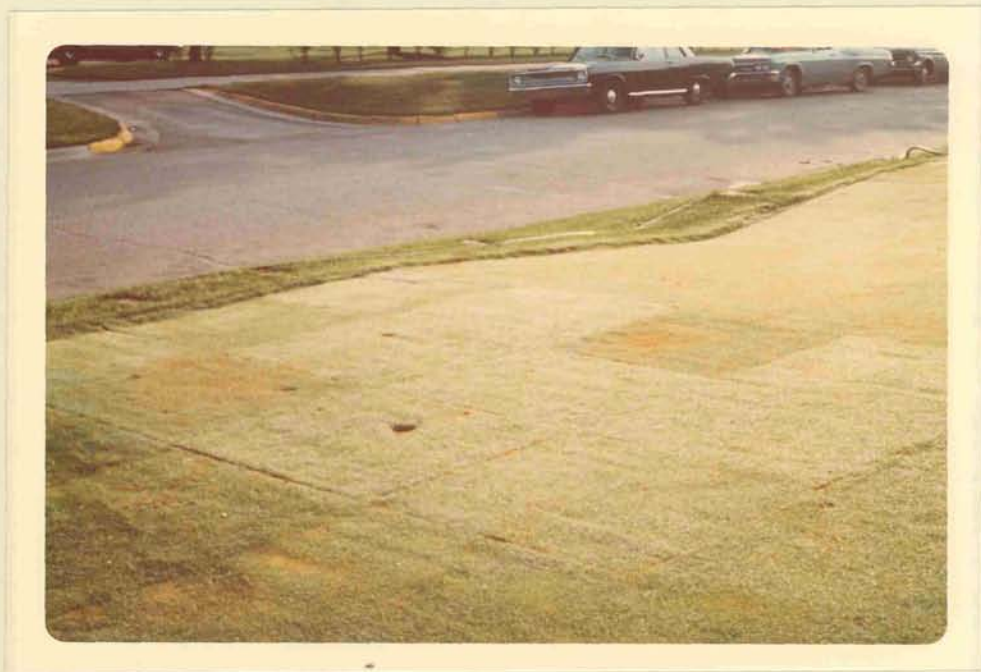
Figure I-6. Morning Dew Pattern of plastic Lined Dune Sand Plots (A) on Ninth Day of the 1969 Dry-down Experiment.
