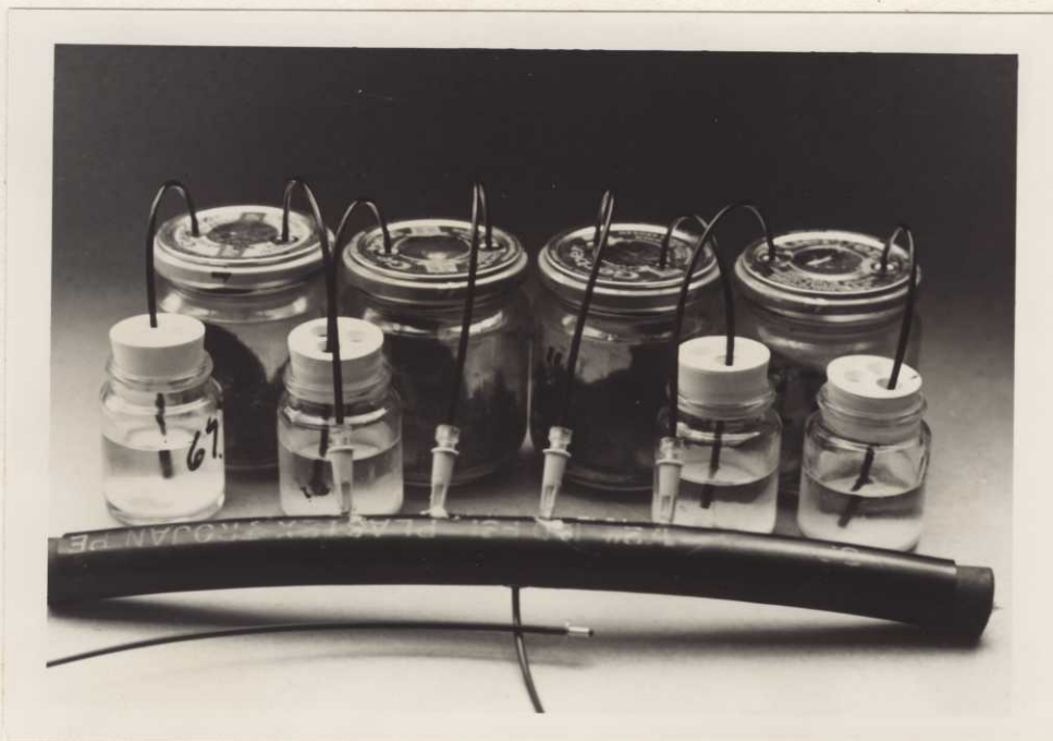
Figure 1. Manifold tubing, incubation jars, and CO 2 collection jars used in the carbon evolution study.
