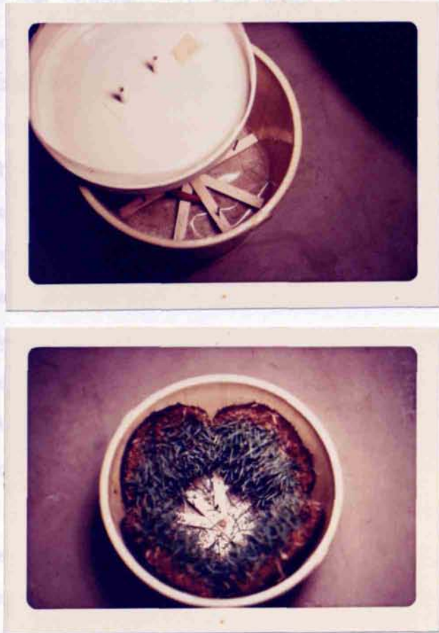
Figure 9. Controlled atmosphere bucket chambers. The lid, gas inlet tube, rack, and arrangement of sod pieces are shown.
