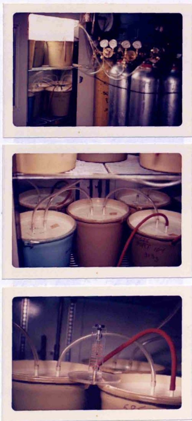
Figure 8. Overall apparatus for controlled atmosphere experiments showing gas delivery and flow metering system.
