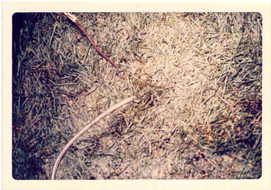
Figure 3. Gas sampling tube, thermocouple, and injured Merion Kentucky bluegrass in the center of the sod piece in a sod heating box are shown.
