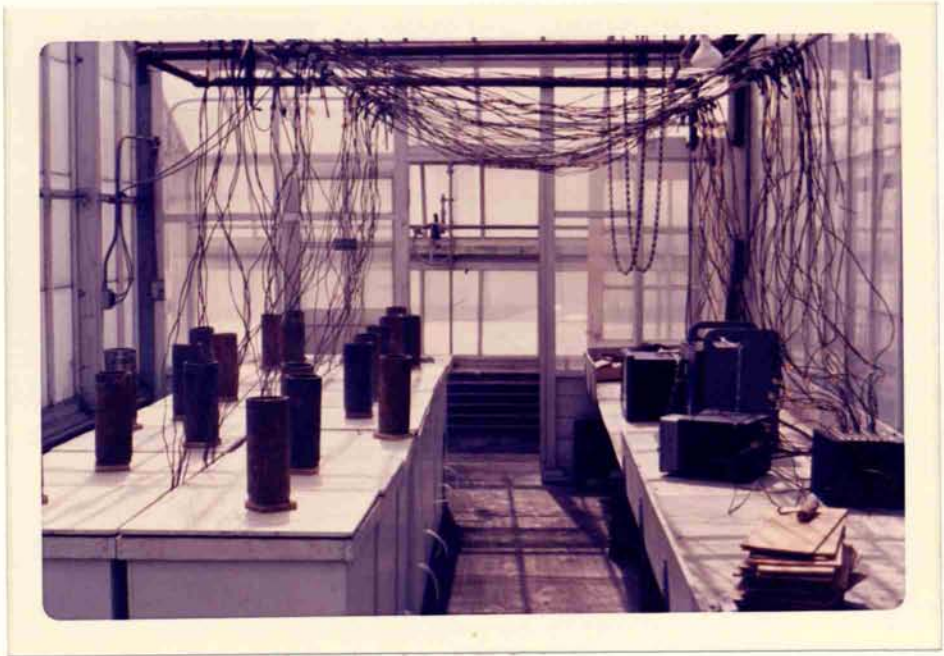
Figure 4. The arrangement of sod heating boxes, weights to hold lids tightly closed, thermocouple wires, recording potentiometers, and protruding gas sampling tubes is shown in the greenhouse room.
