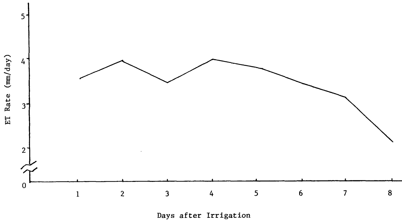
Fig. 8. Changes in the average ET rate for twelve turfgrasses when grown under progressive water stress and uniform cultural practices ( 0.25 kg N are -1 growing month -1 and 3.8 cm cutting height ).
